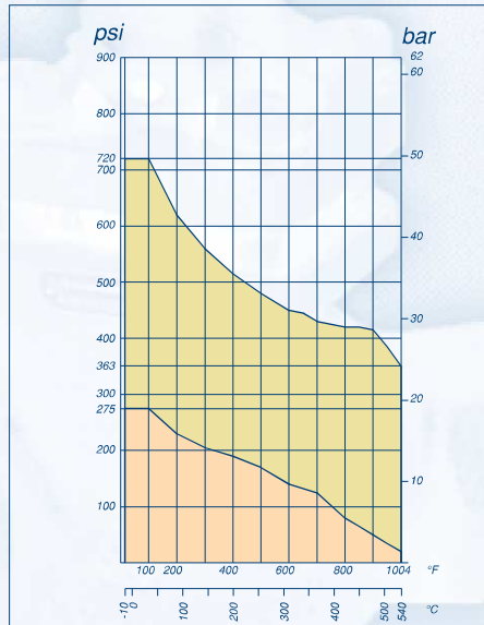
Pressure and temperature limits (A 351 CF8M)
