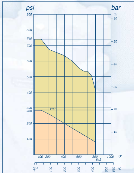
Pressure and temperature limits (A 216-WCB)
